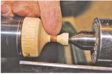
▲ Pic.7 Continue down the sizes, reducing the platens as required until you have a full set of plugs
